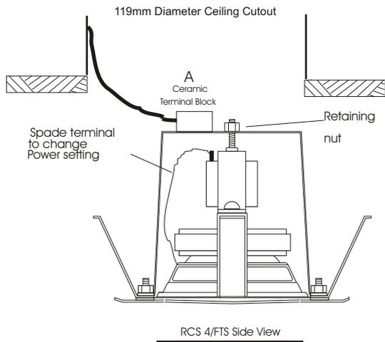
1. Terminate to the ceramic terminal block as shown on the drawing. "A"
