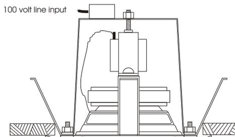
3/ Speaker installed in correct position
