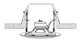
4. Fit second "V" clip into second retaining ears and gently push the speaker up into the bracket (do not push the central perforated grille area) the speaker will self locate into the bracket.
