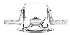
4. Fit second "V" clip into second retaining ears and gently push the speaker up into the bracket (do not push the central perforated grille area) the speaker will self locate into the bracket.
