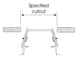
1. Cut the required hole for the speaker
