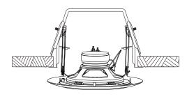
4. Fit second "V" clip into second retaining ear and gently push the speaker up into the bracket (do not push the central perforated grille area) the speaker will self locate into the bracket.
