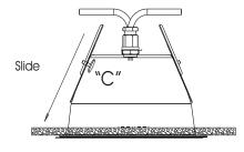
Fitting the dome into a ceiling 7. Loosen the retaining knob for slider "C" Push sliders to the top of the dome and insert dome into pre-cut hole.
