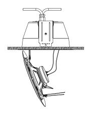
9. Fitting the speaker Compress "V" spring and fit into the retaining ear within the dome. Connect leads to the speaker transformer.
